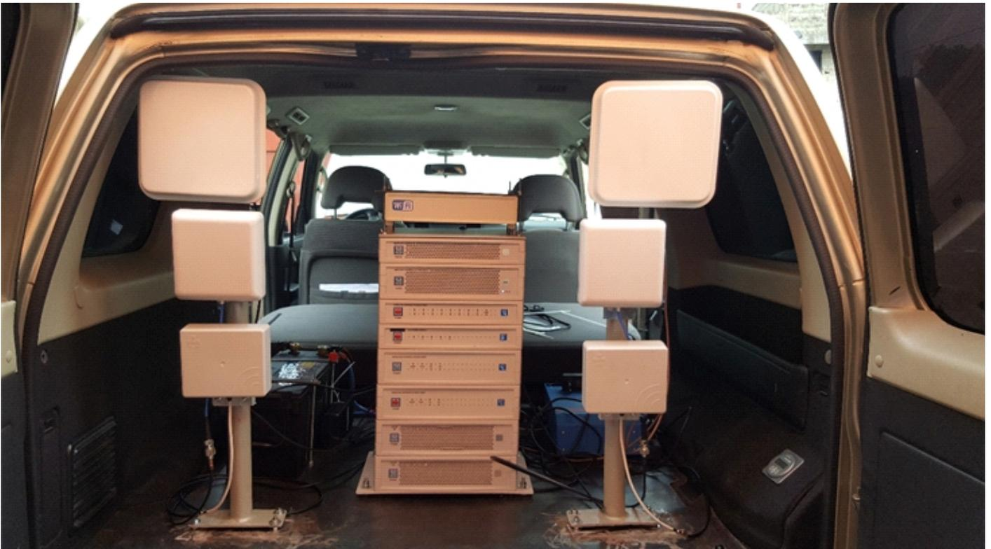
**Above is the actual installation in a vehicle for tactical GSM and WiFi Interception, recording and analysis.**
